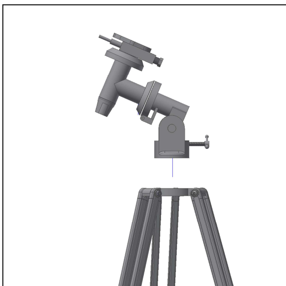
Figure 4. Place equatorial head on top of tripod.
